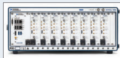
▲ Fig. 2 Compact 8x8 MIMO system with eight VSTs.
